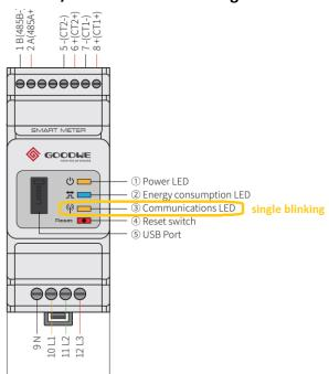
GM1000/GM3000 comes with three LED lights. *The bottom orange light should be single blinking* to indicate the communication with inverter is successful. If blue LED light is off, export limit does not work.
